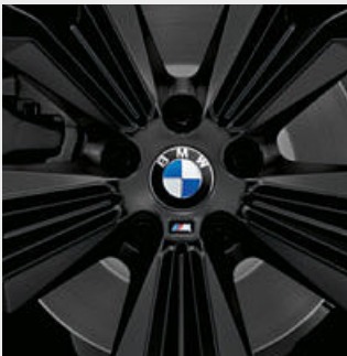
○ The floating hub cap consists of the BMW logo that no longer turns with the wheel but instead remains level.
