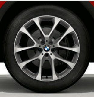
■ 20" light alloy wheels V-spoke style 738 Bicolour Ferric Grey with mixed tyres and runflat properties*, gloss-lathed, front 9J x 20 with 275/45 R20 tyres, rear 10.5J x 20 with 305/40 R20 tyres. 1
