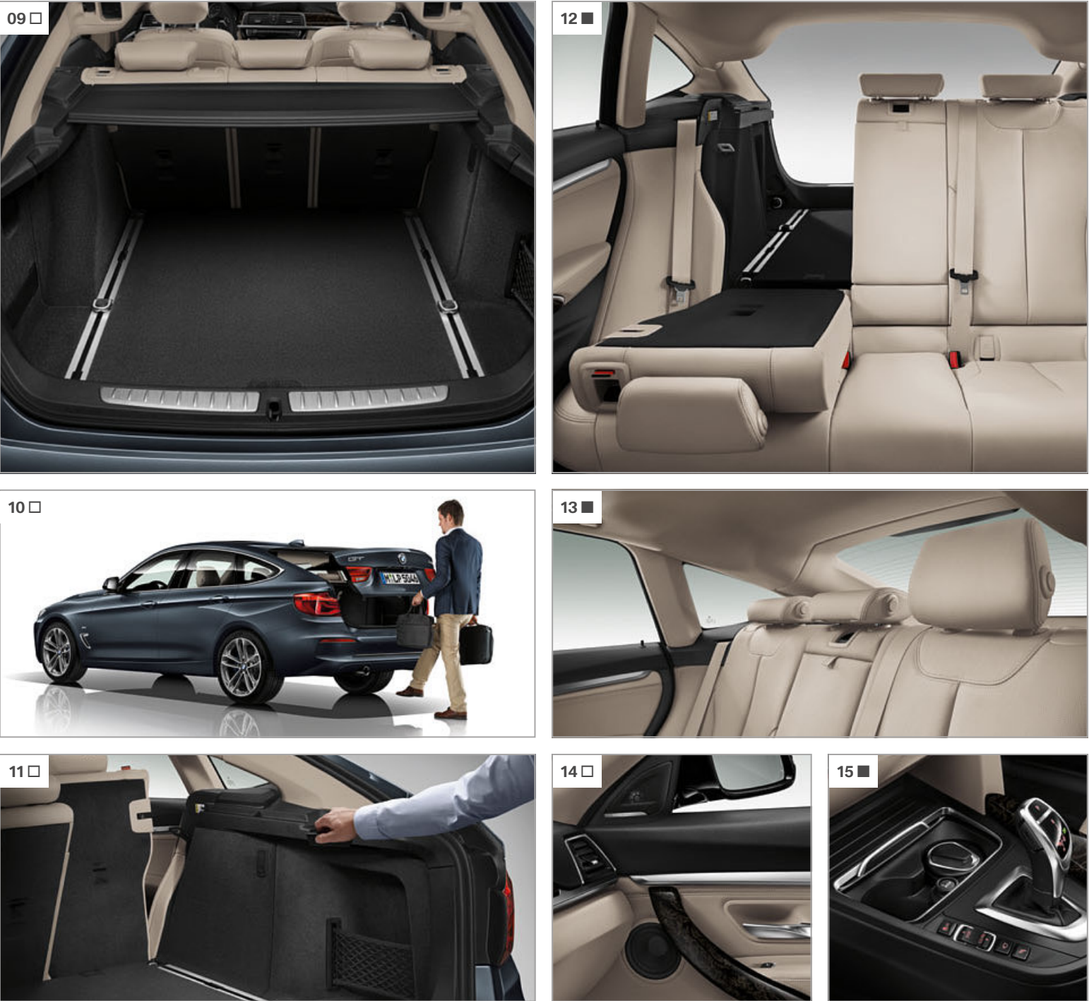
[ 09 ] The Storage compartment package includes items such as practical additional compartments, luggage compartment lashing rails, a storage tray and an additional 12V power socket. 6
