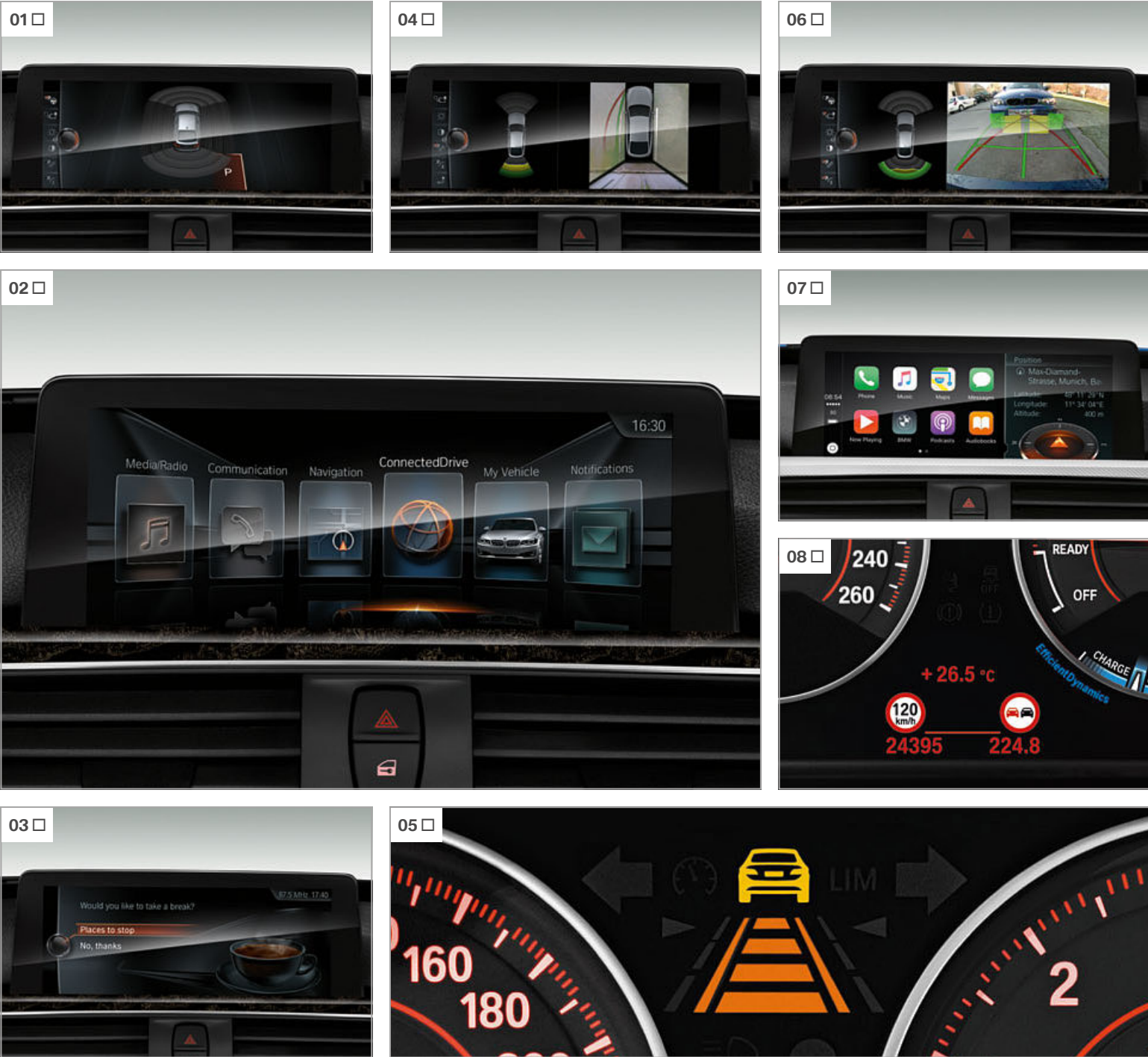
[ 01 ] The Parking assistant makes parking parallel and perpendicular to the road easier. It does the steering while the driver remains in control of the accelerator, brake and gears.
